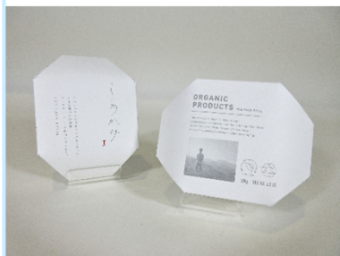
▲ Kome-kami TP-FS, a paperboard made with waste rice, developed jointly with Papal Co., Ltd.
